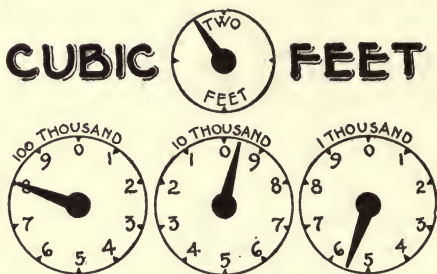
FIG. 42.—Gas meter index reading 79,500 cubic feet.
